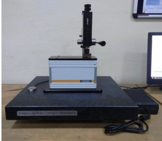
Fig.9 Microhardness measuring machine (Fischerscope instrument).
