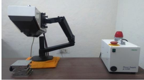
Fig. 4 Residual stress measuring machine
